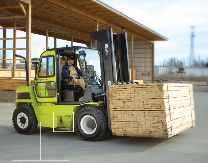
Foot steps with **traction plates** make entry/exit quick, easy and safe... from either side. • The spacious **operator compartment** includes an easy to read color display. Real time information including error codes for the transmission and engine are shown in the LCD display.
